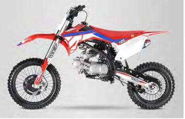
This new 125cc RXF Freeride version was developed based on the RFZ Lwb 2016. In addition to its new plastic kit, the chassis has completely changed with the arrival of its new molded frame feet and brake pedal mounted on bearings that now passe over the footrests. This handy and versatile bike can be used both cross and enduro, so do not hesitate!
